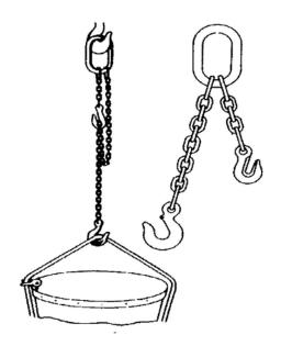
7. Use slings of proper reach. Never shorten a sling by knotting it, or with nuts and bolts. Adjustable slings are available for applications requiring slings of varying reaches
